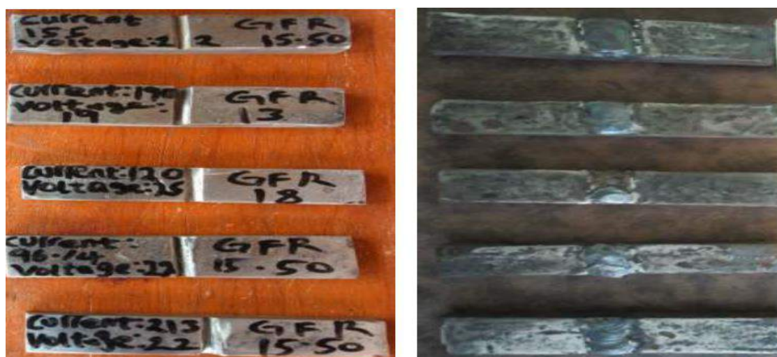
Figure 1: Mild steel samples before and after welding.
