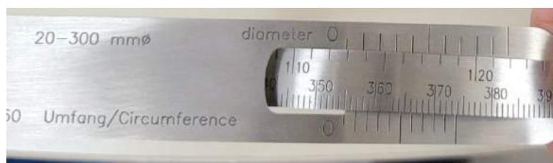
Figure 2. Circometer both measures circumference and diameter at the same time.
