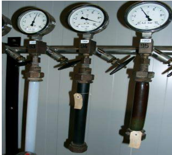
Figure 3. Polyethylene pipes tested since 1957 (Belloir 2008)
