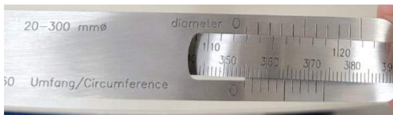
Figure 2. Circometer both measures circumference and diameter at the same time.
