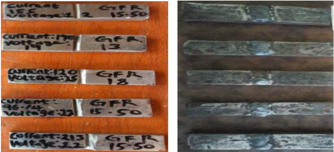
Figure 1: Mild steel samples before and after welding.
